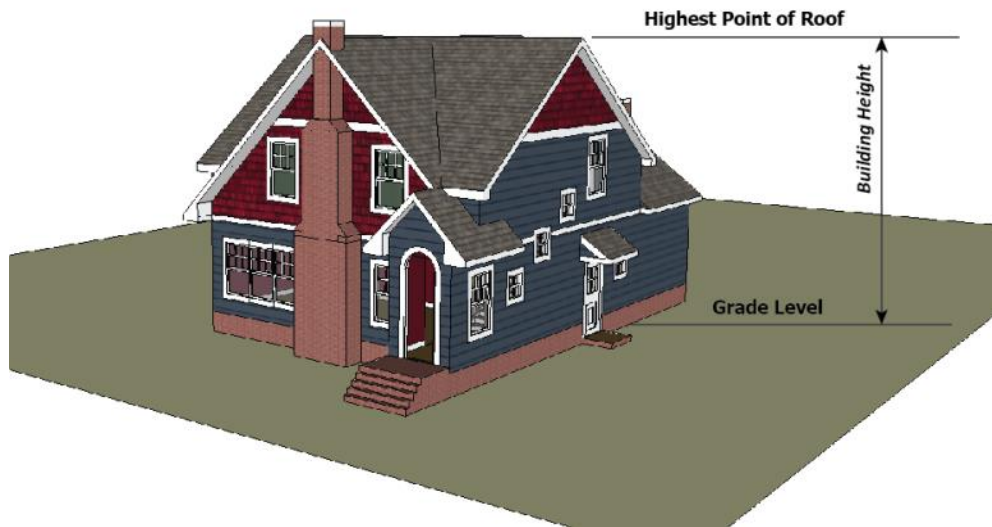
Figure 4.09-J: Measurement of building or structure height
