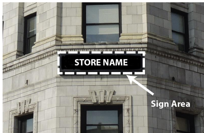
Figure 12.07-C: Illustration of computing the sign area for wall signs with a background panel or cabinet.
